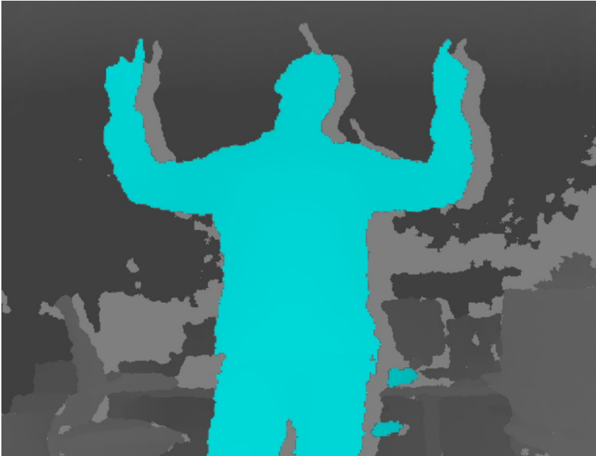
FIGURE 2-3 Depth value samples with player identification.
